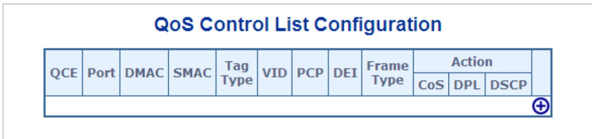
The screenshot shows a table titled "QoS Control List Configuration". The table has columns for QCE, Port, DMAC, SMAC, Tag Type, VID, PCP, DEI, Frame Type, and Action. The Action column is further divided into CoS, DPL, and DSCP. A plus sign icon is visible in the bottom right corner of the table area.
