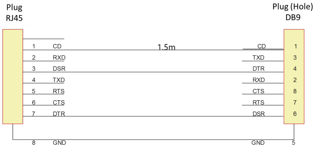
Figure 3- 5 Cable connection at the consoleport
