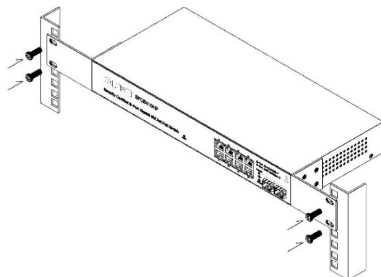
SFC400HP, SFC450HP Rack Mount 장착 모습
