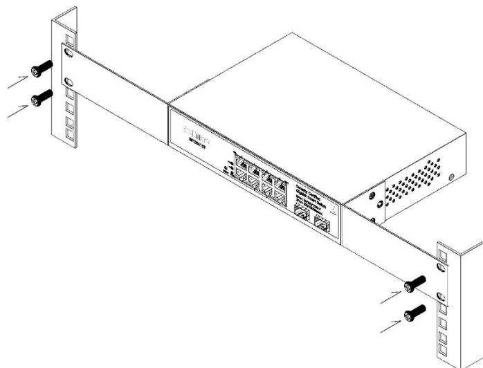
SFC400GM, SFC450R Rack Mount 장착 모습
